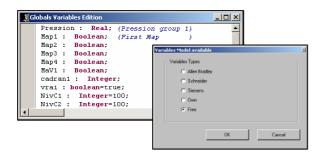
A simple grid of parameter setting, allows to carry out the link between the global variables and the remote I/O. This software allows to test the communication and to visualize the state of the inputs/outputs.
