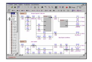
Visual PLC has a complete library of functional modules which you can enrich. In the editor of functional modules, you will define the parameters of entry and exit and the source code of your module.
